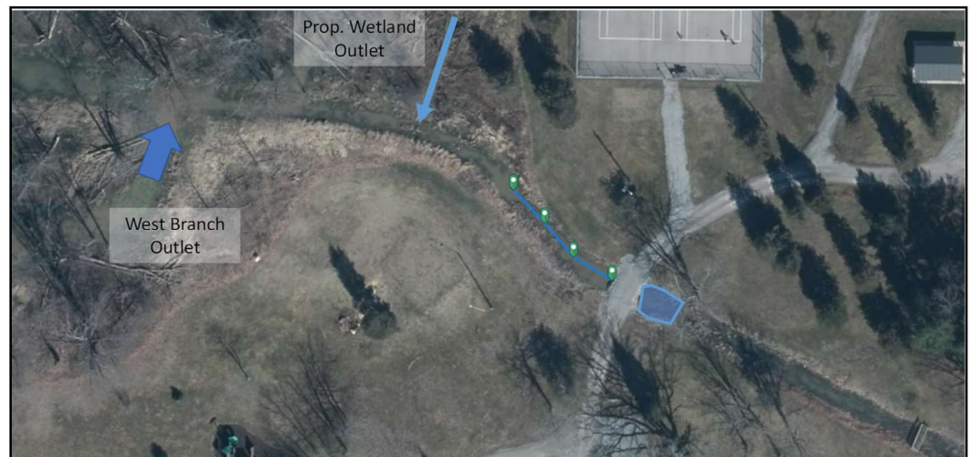
Figure 9 Centennial Park Culverts Proposed Riffles and Pool
