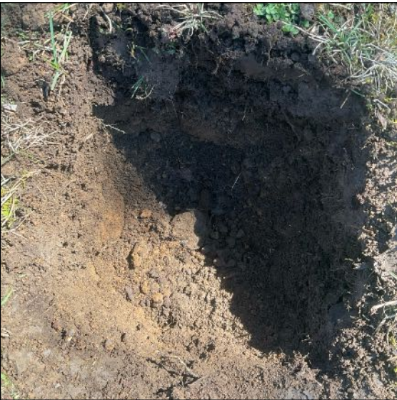
Image 5: Example of disturbed Test Pit conditions. Note lack of topsoil.
